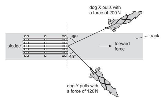
Dog X pulls with a force of 200 N at an angle of 65° to the front edge of the sledge. Dog Y pulls with a force of 120 N at an angle of 45° to the front edge of the sledge.
